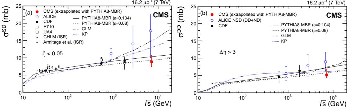
**Figure 1:** Measured SD (left) and DD (right) cross sections for  $\xi < 0.05$  compared with theoretical predictions. The model embedded in PYTHIA8-MBR provides a good description of all data.
