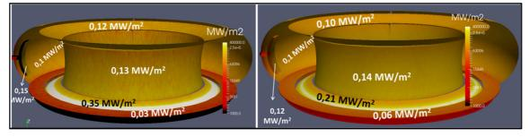
Figure 2: Radiative power loading (6MW core + 4 MW divertor plasma). Left: R=0 Right :R~0,5
