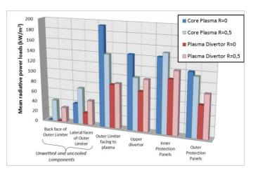
Figure 3: Mean radiative power load for 10MW divertor plasma (red) and core plasma (blue)
