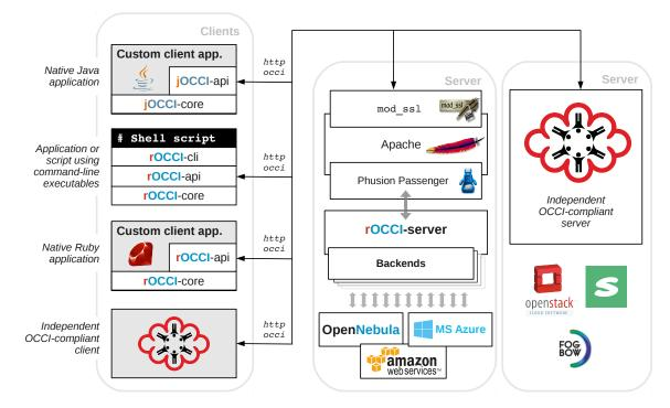
Figure 2: Various OCCI implementations on both the client and the server side, communicating over HTTP/OCCI
