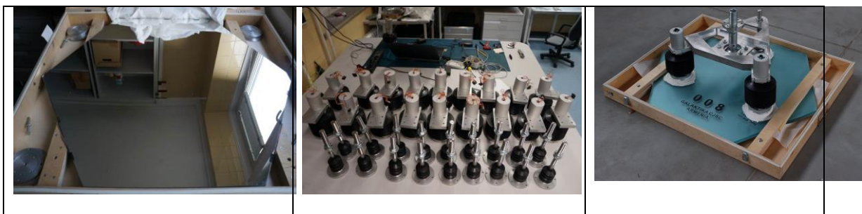
Figure 6 Manufactured components of SST-1M Optical systems: glass mirror facet (left), actuators (middle), integrated mirror alignment fixing set (right)
