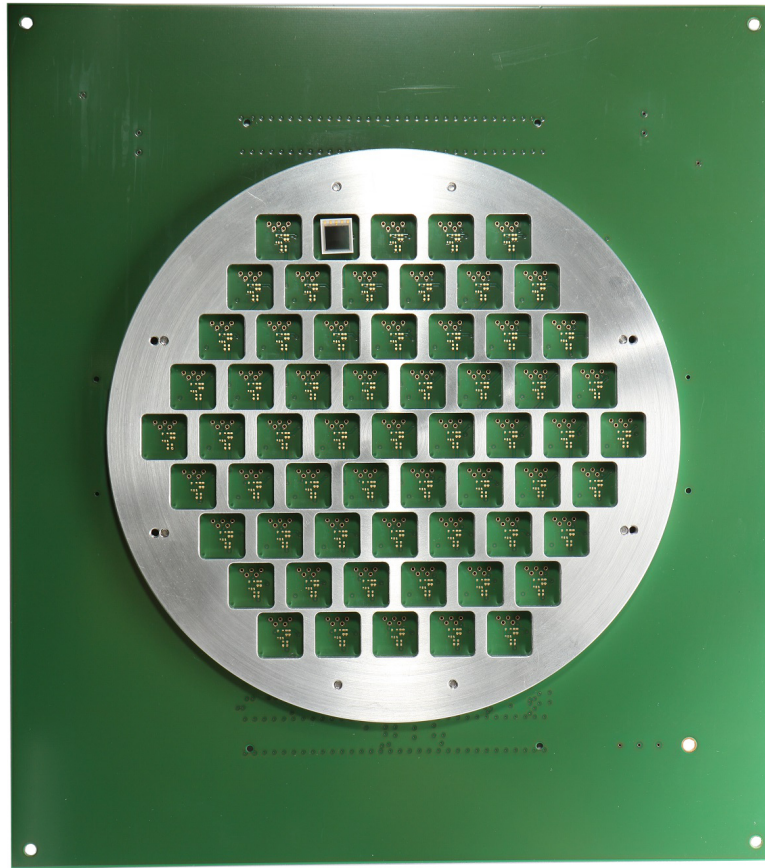
Figure 4: The new focal plane of the FAMOUS telescope. Visible is the PCB which will host the 64 SiPMs and an aluminum grid into which the 61 Winston cones will be glued. As an example one SiPM is shown. The three blind pixels are hidden by the aluminum border.
