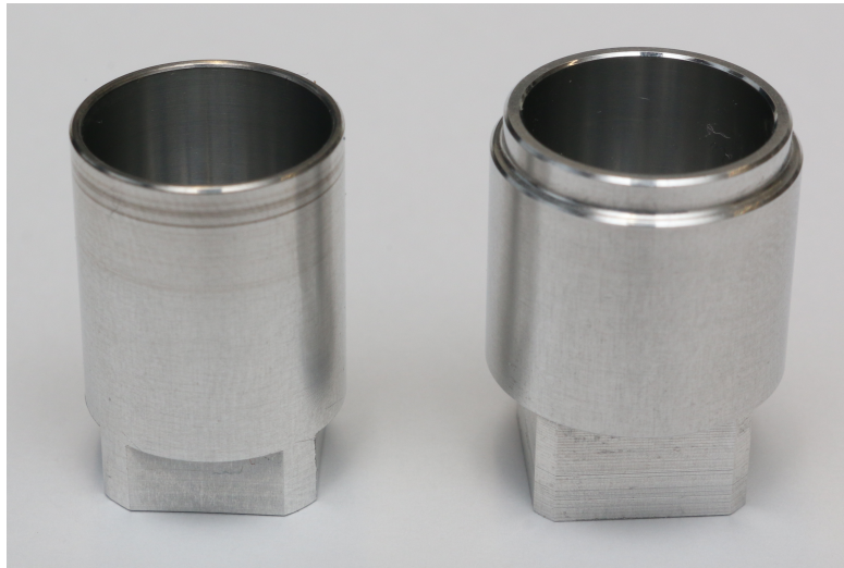
Figure 3: A comparison between the old Winston cone with an additional edge for assembly (right) and the new one with a smaller rim (left). The inner geometry is identical
