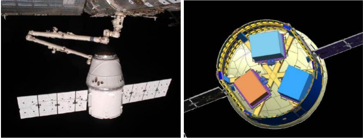
Figure 1: The Dragon spacecraft of SpaceX at the ISS (left) and the unpressurized part of the craft's payload bay (right) [7, and references therein].
