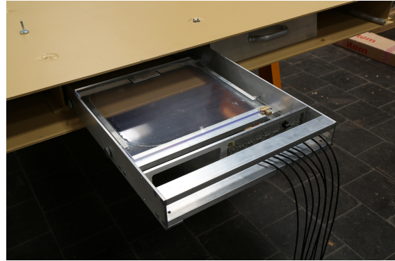
Figure 3: Photo of a scintillator tile with optical coupling between WLS and clear fibre. The WLS fibre is glued into the scintillator groove.
