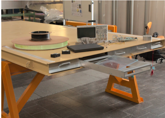
Figure 2: The AMD detector prototype. Shown is half of the steel housing with 32 scintillating tiles in 4 trays.
