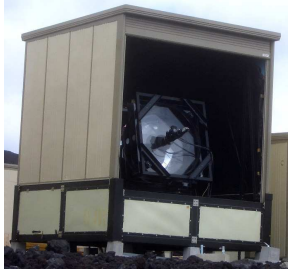
Figure 2: An Ashra-1 light collector.
