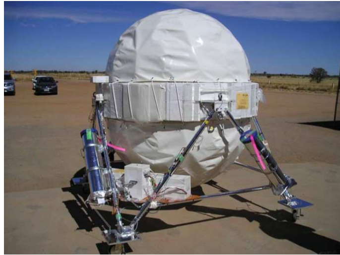
Figure 2: GRAINE-2015 balloon-borne gondola before launching. One of three star cameras was set on the opposite in this picture.
