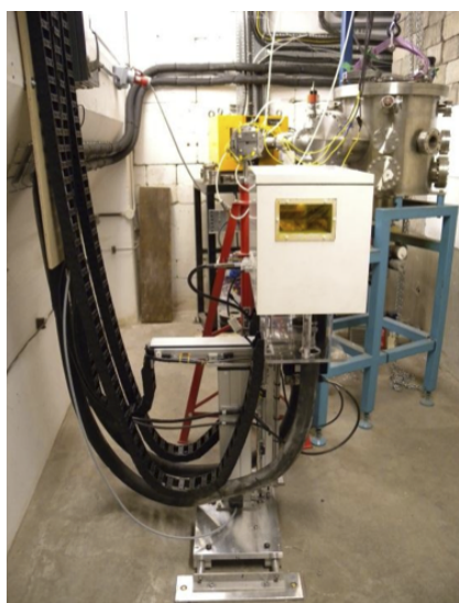
Figure 2: The pre-configured XY-axis Cartesian robot system and cool box within the high intensity irradiation area at the Medical Physics MC40 cyclotron, University of Birmingham
