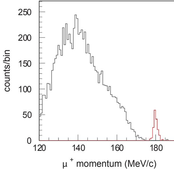
**Figure 3:** Monte Carlo simulation of the  $\mu^+$  momentum distribution in E36 with  $K_{\mu 3}$  spectrum (black) and  $K^+ \rightarrow \mu^+ N$  spectrum (red) assuming  $BR(K^+ \rightarrow \mu^+ N) = 2 \times 10^{-8}$  and  $M_N = 220 \text{ MeV}/c^2$ .
