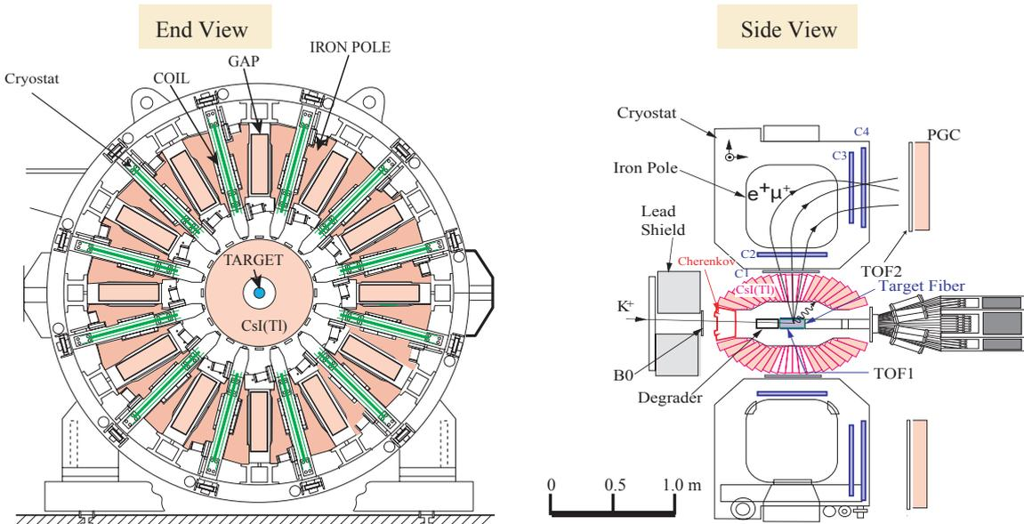
**Figure 1:** Schematic view of the TREK detector for experiment E36 [5] after upgrade from the KEK E246 apparatus.
