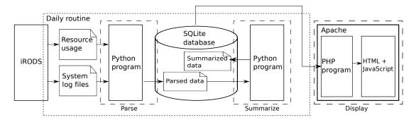
Figure 2: SCALA workflow in iRODS
