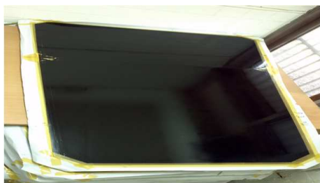
Figure 5: Photograph of a completed HPL gas gap at Kodel.
