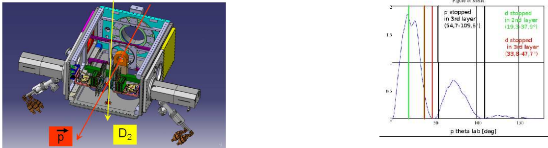
Figure 7: Left panel: Experimental setup for the measurement of the beam polarization as it was used during the beam time. The cluster target beam comes from the top and crosses the polarized proton beam stored in the machine. Elastically scattered deuterons are detected two silicon telescopes. Right panel: FOM for the polarized of the elastic reaction as a function of the deuteron scattering angle. Both p and d ejectiles are detected in the telescope system.
