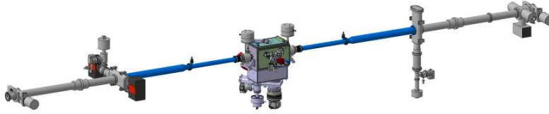
Figure 5: Overall view of the vacuum setup at the PAX interaction point. The NEG coated tubes are indicated in blue. The measured beam-lifetime during the spin-filtering cycles was > 6000 s, exceeding the expectations and allowing for longer spin-filtering cycles than initially planned.
