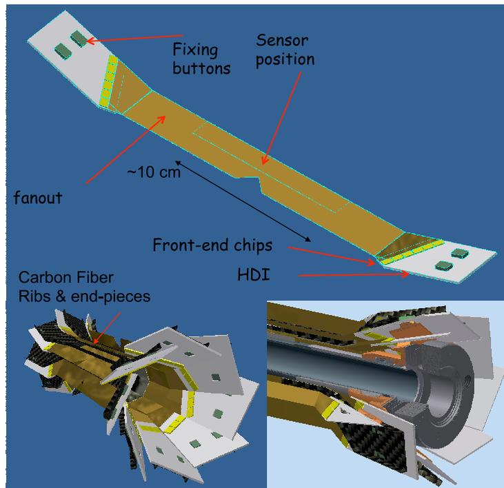
**Figure 2:** Drawings of the octagonal Layer0 made of stripsets modules. In the inset, the stripset modules positioned on the cold flanges with the Be beam-pipe.
