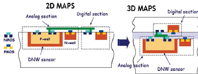
**Figure 4:** Schematic concept of 2D MAPS, with DNW sensor on a single CMOS tier, and 3D MAPS realized with two CMOS tiers interconnected.
