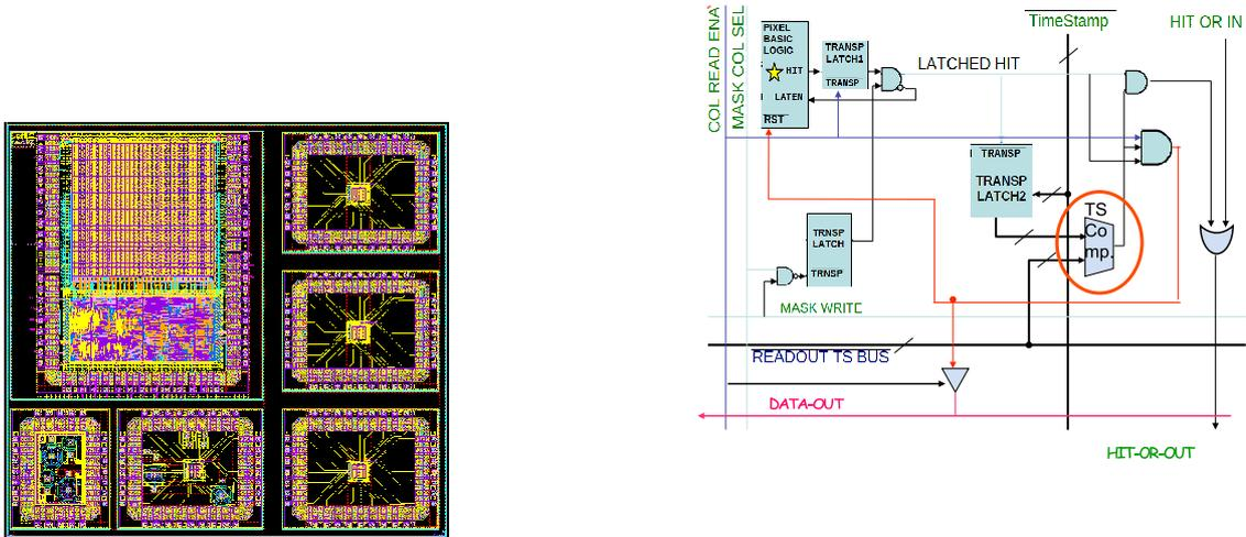
**Figure 3:** Left: the layout of the chip submitted in the INMAPS, with the 32x32 pixel matrix and the other test-structures. Right: schematic of the in-pixel logic needed for a time-ordered readout.
