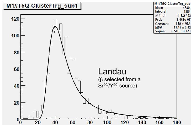
Figure 5: Cluster signal of the 3x3 MAPS matrix with a  $^{90}\text{Sr}$   $\beta$  source.
