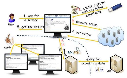
Fig. 1 – Accessing the Grid infrastructure with the GENIUS portal and certificates on smart cards.
