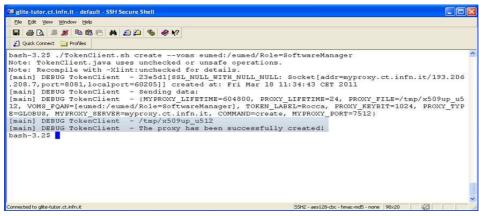
Fig. 5 – The TokenClient sends a "create" request to the eTokenServer.
