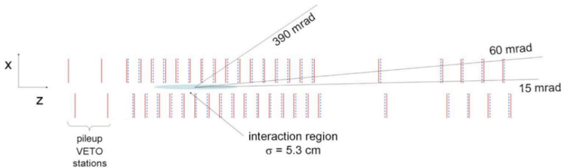
**Figure 1:** Schematic of the two VELO halves, as seen from above. The two rows consist of 21 modules, where each module is made up of two silicon sensors mounted back-to-back. The VETO or pile-up stations are seen on the left. As a detector safety consideration, the VELO halves are retracted during beam injection and adjust, but closed around stable beams. The right handed co-ordinate system is shown.
