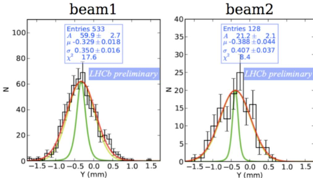
**Figure 8:** The measured beam sizes (red), and the vertex resolutions (green) for beam 1 and beam 2. The resolution is unfolded from the measured size to give the bare beam profile (yellow - close to the red).
