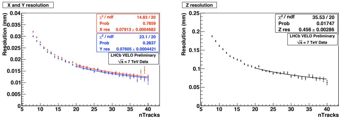
**Figure 6:** Resolutions as a function of track multiplicity in data. The data points are fitted between 20 and 40 tracks with the function  $\sigma_{res} = \sigma_0/\sqrt{N}$ , where  $\sigma_0$  is the fitted constant and  $N$  is the number of tracks.
