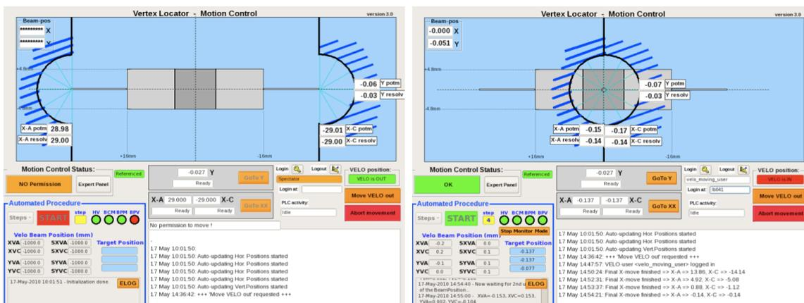
**Figure 2:** Screenshots of the PVSS closing manager, showing the VELO in the retracted position (left) and then after closing (right). This panel updates in real-time during the closing procedure.
