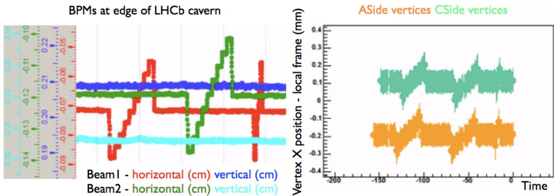
**Figure 4:** During a Van der Meer scan, the movement of the two beams in the horizontal plane (seen in the BPMs, left) manifests itself as a change in the x position of the reconstructed vertices (right). The offset between A and C side vertices is due to measurements being made in the local frame of each half.
