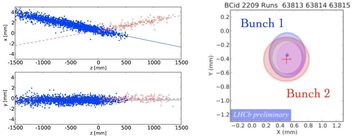
**Figure 7:** Left: Scatter plot of beam gas events reconstructed by the VELO in the longitudinal  $(x,z)$  and  $(y,z)$  planes. Blue shows beam 1, red beam 2. The crossing angle is clearly seen. Right: Measured  $1\sigma$  contour of each beam at the interaction point, shown in the  $(x,y)$  plane. The measured luminous region is shown in purple, and the predicted luminous region white.
