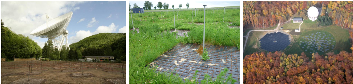
Figure 1: Left: LBA field of the Effelsberg station with the 100 m radio telescope in the background, centre: LBA antennas in Unterweilenbach, right: the Tautenburg station with HBA and LBA fields and the dome of the 2 m optical telescope.
