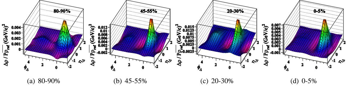
**Figure 13:**  $p_t$  correlations for 200 GeV AuAu collisions for various centralities. These correlations have been inferred from the inversion of scaled fluctuations and we have subtracted the multipoles. The shapes of the peaks at  $(0,0)$  are different than those of number correlations and there is a “recoil” hole around the peak.
