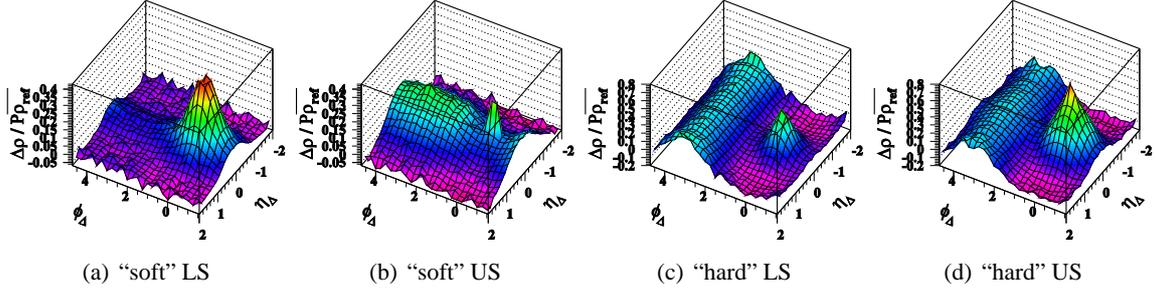
**Figure 5:** Projections of two-particle correlations onto  $(\eta_\Delta, \phi_\Delta)$  space with cuts on  $(y_{t1}, y_{t2})$  space. Soft pairs have  $y_{t1} + y_{t2} < 2.7$  and hard pairs  $y_{t1}, y_{t2} > 2$ . For the soft pairs the LS has a strong HBT component while the US is dominated by local measure conservation such as momentum and charge. For the hard pairs the AS ridge is charge independent while the SS jet peak is primarily US.
