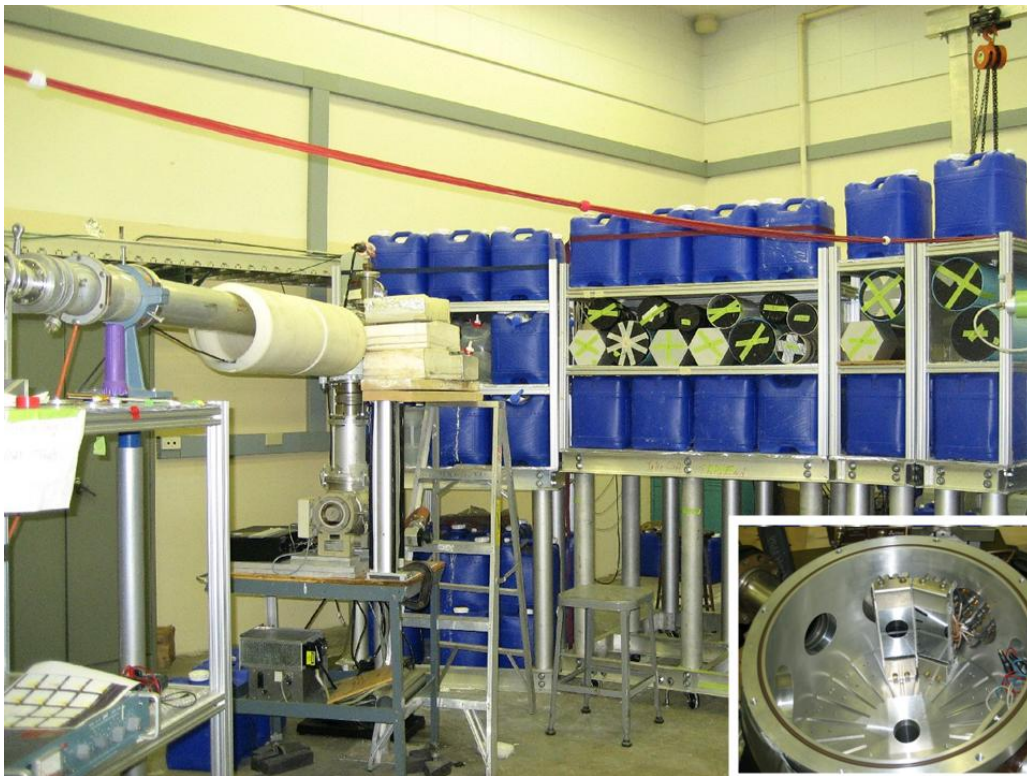
Figure 2: Array of 16 neutron detectors located at 3.6 meters away from reaction chamber. The insert in the lower right shows the reaction chamber with the silicon detector array.
