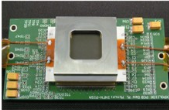
Figure 5: the sealed Gas Pixel Polarimetric Detector with the 50 nm Be window [7].
