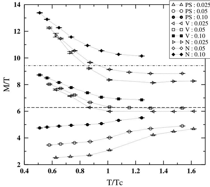
**Figure 1:** The screening masses of pseudo-scalar (PS), vector (V) mesons and nucleon (N), divided by the temperature  $T$ . The dashed (dot-dashed) line represents the free-quark limit  $2\pi$  ( $3\pi$ ).
