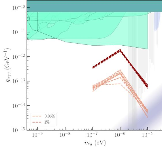
**Figure 3:** Estimated sensitivity of current radio telescopes to the spectral radio feature produced by resonant photon production from axion clouds. For reference we also show the parameter space for the QCD axion (purple), and current constraints from astrophysical searches (light green and light blue), axion haloscopes (grey), and heliscopes (dark green). See [15] for additional details.
