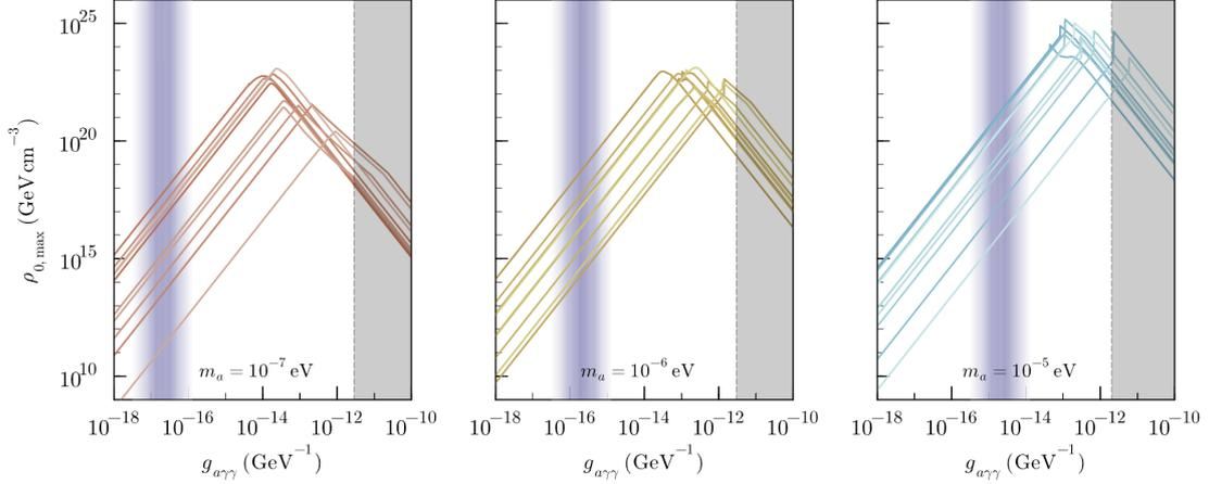
**Figure 2:** Maximal density of the axion cloud for each neutron star in our sample as a function of axion-photon coupling and axion mass. The QCD axion parameter space is shown in purple, and current excluded parameter space is shown in grey [13].
