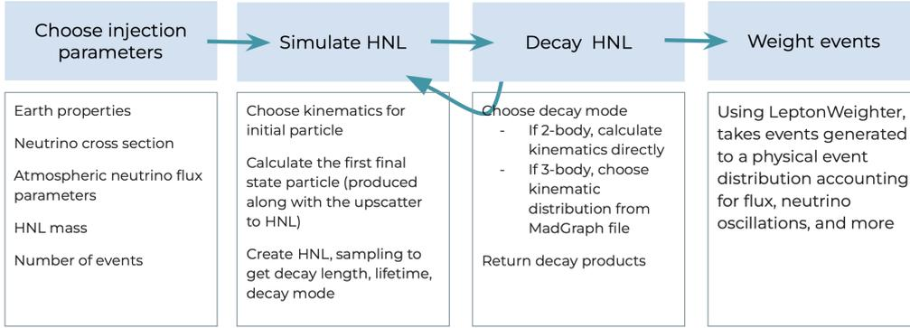
**Figure 3:** Flowchart describing the process of simulation procedure for HNL events with LeptonInjector-HNL.
