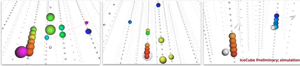
**Figure 2:** IceCube low-energy event morphologies from simulation. From left to right: track, cascade, double cascade. The magenta ball and arrow in the leftmost plot indicates the origin point and direction of the track, while the red to blue color scale of other bubbles indicates photon arrival time at each DOM, with red corresponding to earliest times. Bubble size corresponds with the amount of light received at each DOM.
