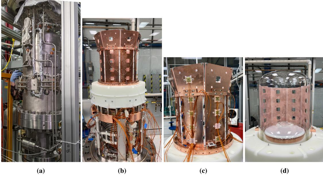
**Figure 1:** (a) SBC-LAr10 pressure vessel. (b) SBC-LAr10 inner assembly with partial insulation. (c) with SiPMs installed. (d) view of the jars.
