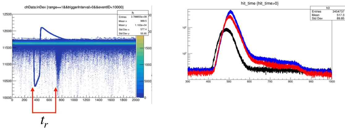
**Figure 3:** Left:Raw waveforms together with the trigger of the optical calibration systems. Marked is the run time between trigger and the acquired PMT pulse. Right:Hit time study of the detector with a small volume of LS encased in a glass bulb positioned at different heights (red and blue) inside the detector vs. natural radioactivity (black).
