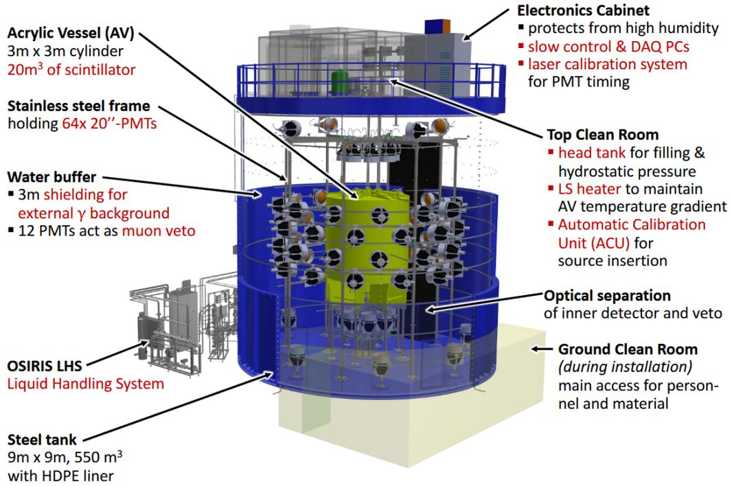
**Figure 2:** The OSIRIS detector as installed in the underground liquid handling hall of JUNO.
