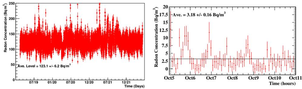
**Figure 1:** The left plot shows the radon levels in the underground SNOLAB laboratory air. The right plot shows the radon levels in the SNOLAB compressed air supply.
