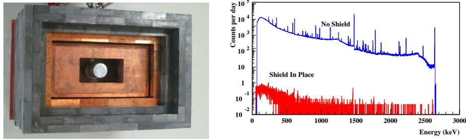
**Figure 2:** The left figure shows the SNOLAB VdA germanium counter, the high purity lead and copper shielding is shown surrounding the germanium detector. The right plot shows the gamma background spectra in the underground laboratory with respect to the fully shielded gamma spectra.
