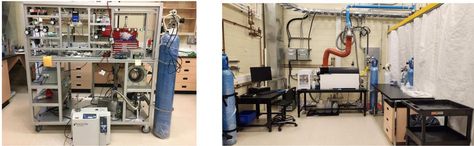
**Figure 3:** The left photo shows the new SNOLAB radon emanation chamber located in the SNOLAB surface laboratory. The right photo shows the new Agilent ICP-MS system in the SNOLAB surface laboratory.
