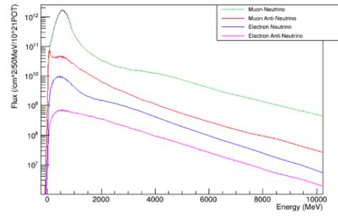
**Figure 4:** JNUBEAM neutrino fluxes at ND280 for a horn current of 250 kA. From webpage: [https://t2k-experiment.org/result\\_category/flux](https://t2k-experiment.org/result_category/flux) (neutrino beam flux prediction 2020).
