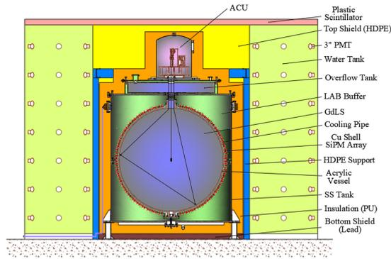
**Figure 2:** Scheme of the TAO detector.
