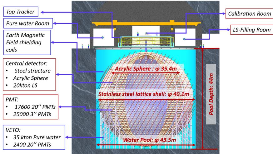
**Figure 1:** The scheme of the JUNO detector.
