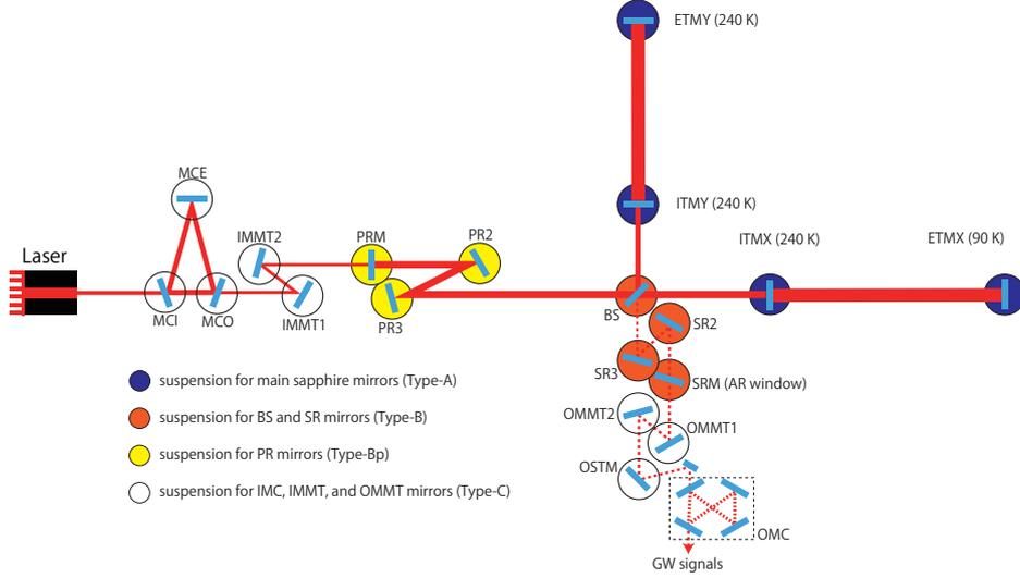
**Figure 1:** Schematic of interferometer configuration during O4 observing run. ETMX was cooled at 90 K and the other sapphire mirrors were at 240 K during the O4. SRM was replaced from 70% reflection mirror to AR coated window to increase GW signals with PRFPMI configuration.
