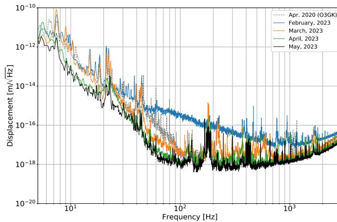
**Figure 2:** Sensitivity evolution of KAGRA after February 2023. Gray dashed lines show the reference sensitivity during the O3GK. Blue lines show the sensitivity when PRFPMI was first locked with DC readout after hardware updates. Orange lines show the sensitivity after reducing MICH, PRCL, and environmental noises. Green lines show the sensitivity with ADSs and WFSs. Black lines show after implementing all ASCs.
