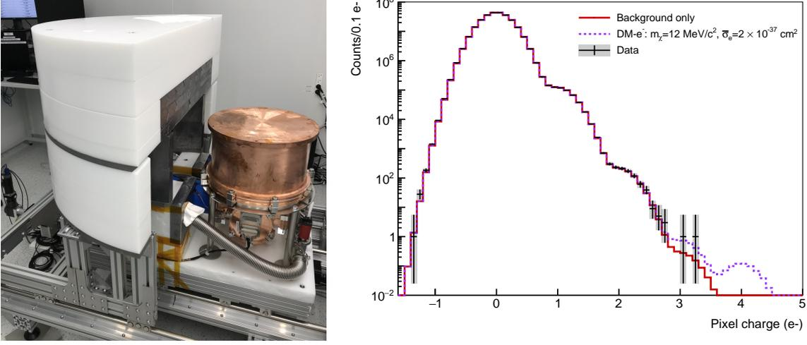
**Figure 2:** Left: The Low Background Chamber at the LSM, outside the movable shielding (half of it visible.) Right: Pixel charge distribution with peaks corresponding to individual charges. The red line is the fit result for the background-only hypothesis (no DM- $e^-$ ). The dashed violet line is the expectation for background plus a DM- $e^-$  heavy-mediator model with  $m_\chi=12$  MeV/ $c^2$  and cross section equal to our 90% CL limit value obtained at this mass.
